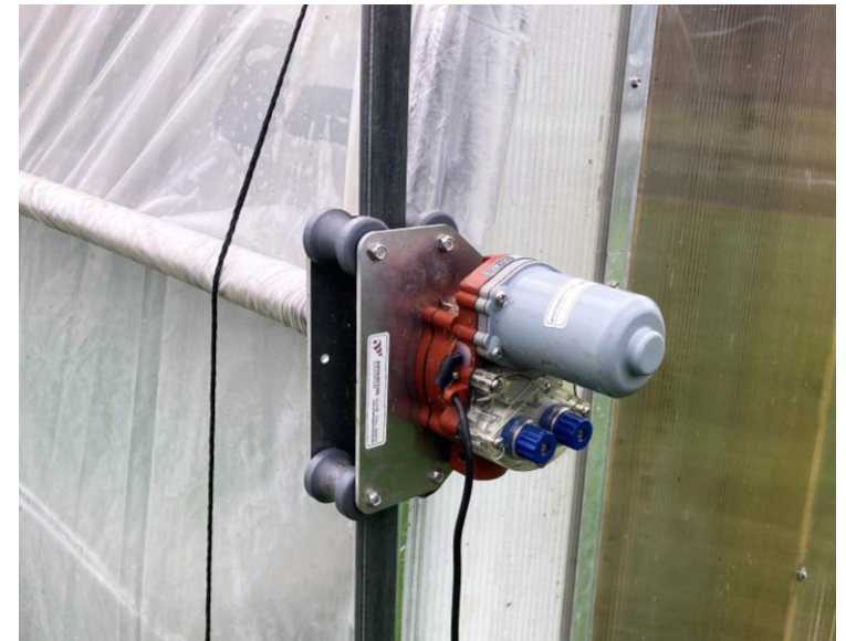
automatic side venting add ~$ 3,000 for two drive motors, controller, thermostat
