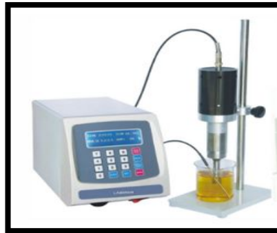
Sonication (High energy method)
