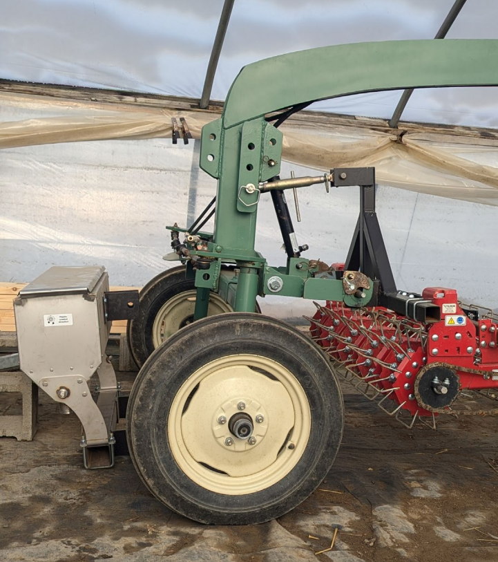
Showing offset steering and fertilizer sidedresser
