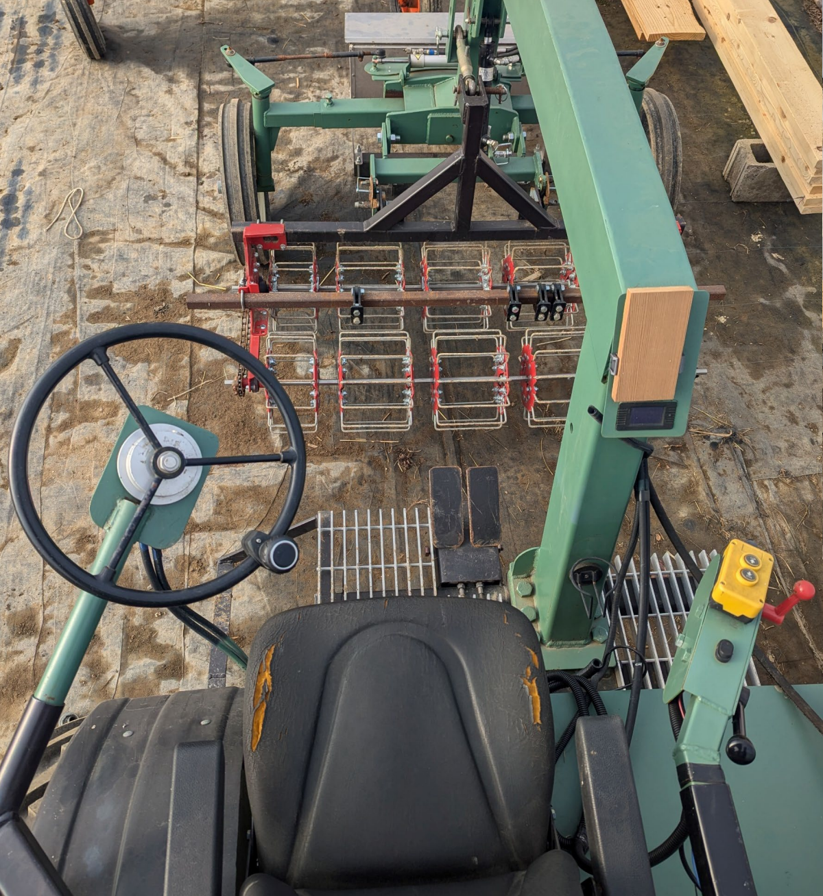
Showing offset steering and fertilizer sidedresser
