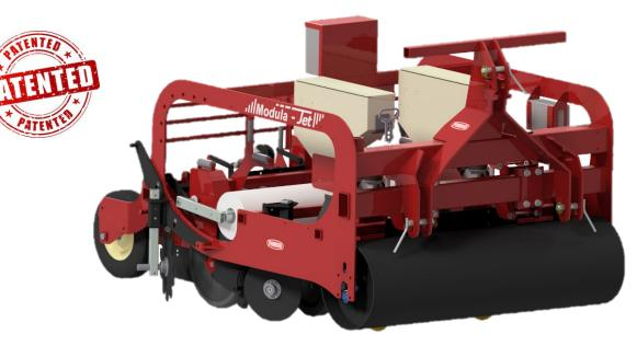
**Modula Jet** is a complete system that allows to lay the plastic film down and seed through it.
