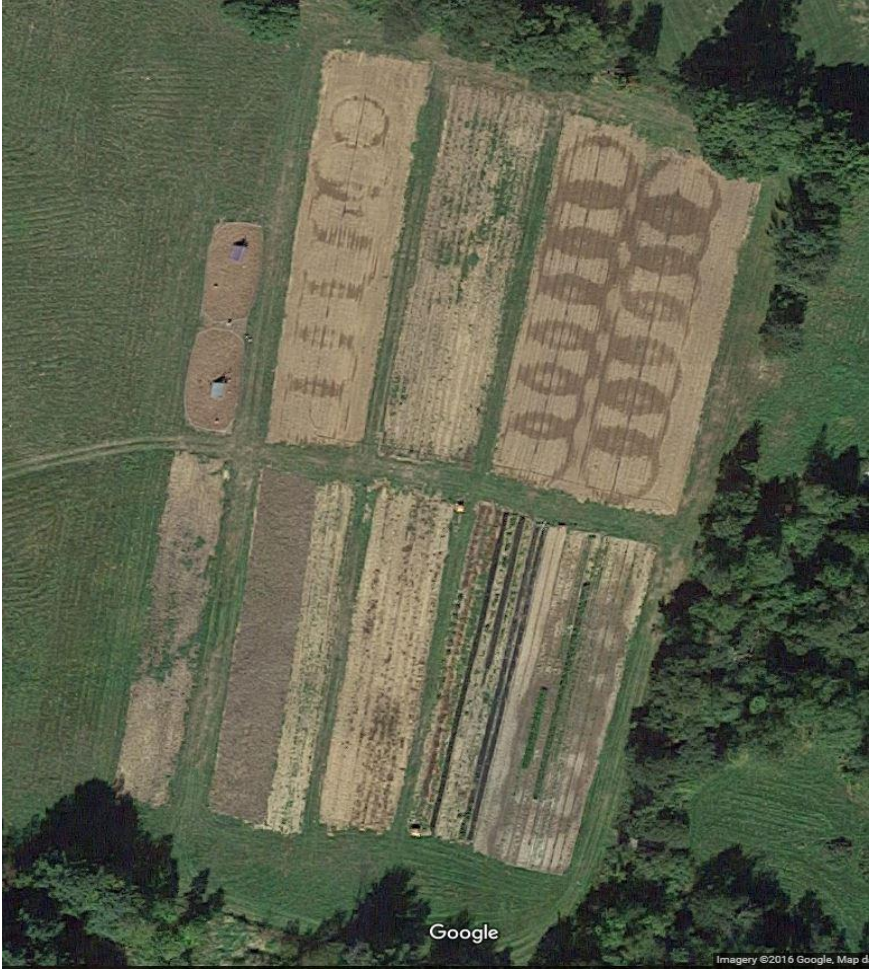
Low application uniformity resulting in dry spots and “doughnut” shaped wet pattern on highly efficient MegaNet rotator system.
