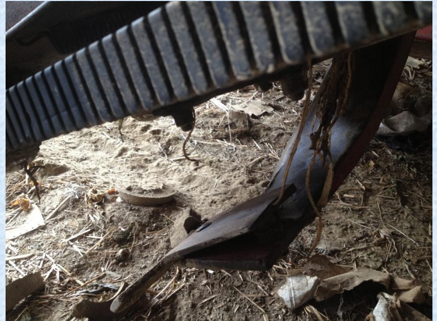
Under cutting plow share and pick up belt
